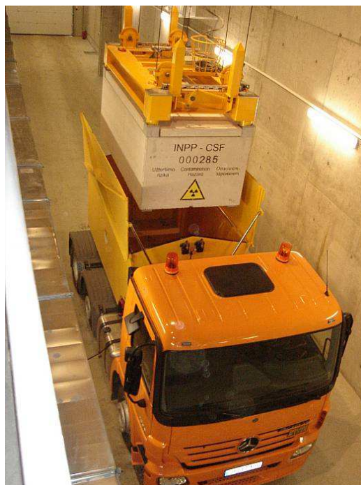
Figure 2.2.5-5. Waste package unloading from truck in room 103
